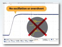
Output voltage waveform with 400 µF capacitor connected
