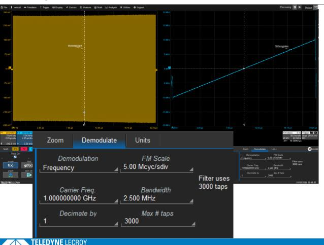
Linear swept sine, is a linear frequency modulates CW. Setting the correc FM demodulation parameter we can see if the FM is linear as expected or not
